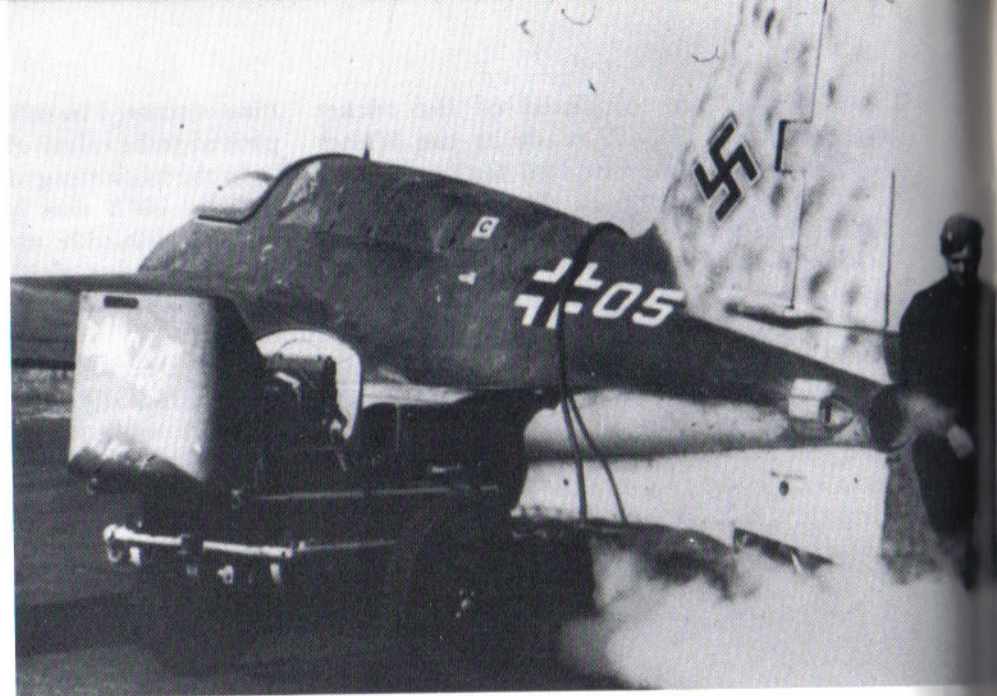
Above right: Starting of the steam turbine which would drive the pumps that would circulate the fuel for the aircraft. The accompanying steam can be clearly seen in the picture.
