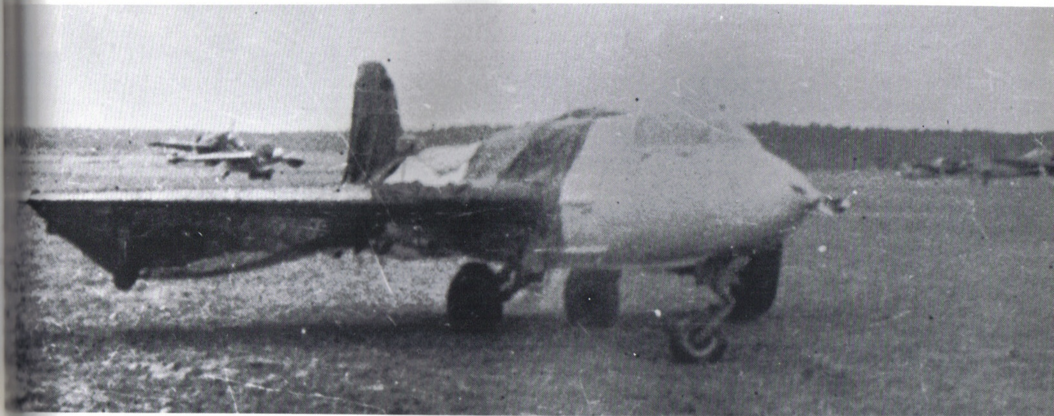
Test example of the Me 163B with lengthened fuselage and nose wheel for early testing of the 263. The lower part of the fuselage shows strengthening rods. In the background an Me 163A.
